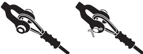
**6** THREAD CABLE THROUGH CHETCO TROLLEY AND A CABLE CLAMP. WRAP CABLE AROUND ANCHOR AND THREAD BACK THROUGH CLAMP.
