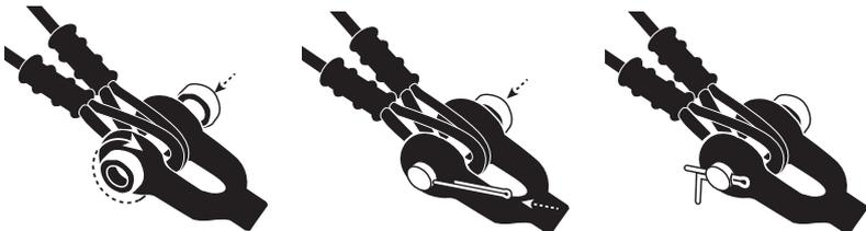
**5** PLACE THIMBLE-END OF MAIN CABLE INTO OTHER TURNBUCKLE JAW. SECURE BOLT WITH NUT OR COTTER PIN. USE A WRENCH TO TIGHTEN NUT. USE PLIERS TO BEND COTTER PIN.
